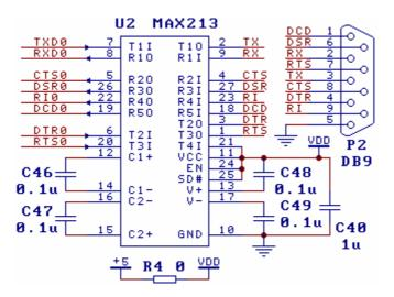
CH342F provides common UART signals and MODEM signals. In the figure, one path of TTL serial port is converted to RS232 serial port through the external level conversion circuit U2. The other path is similar. Port P2 is a DB9 pin, and its pins and functions are the same as those of the ordinary 9-pin serial port of the computer. The similar models of U2 include MAX213/ADM213/SP213/MAX211. USB bus uniformly supplies power to U2 in the figure through R4.
