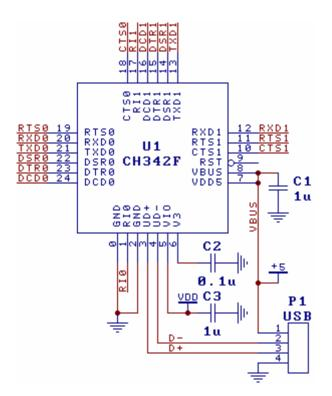
The figure above shows the USB to dual TTL serial ports realized by CH342F. The signal wires in the figure can only be connected to RXD, TXD and the common ground wire. Other signal lines can be selected as needed, and can be suspended when not needed.
