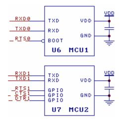
The figure above shows the reference circuit of MCU connected to CH342 chip through two TTL serial ports to realize USB communication under dual power supply mode. CH342 is powered by USB bus. Another self-supplied power VDD is used for VBUS, MCU1, MCU2 and VIO. VDD supports 5V, 3.3V, 2.5V and 1.8V.
