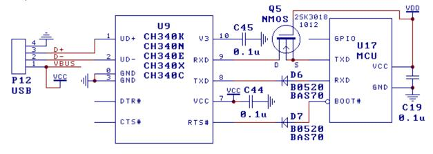
7.7 Connect to MCU, Supply Power to Each, and Prevent Flooding in Both Directions (Figure Below)
