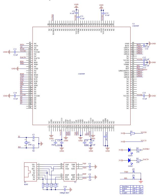
Figure 9-2 CH395P Hardware reference circuit
