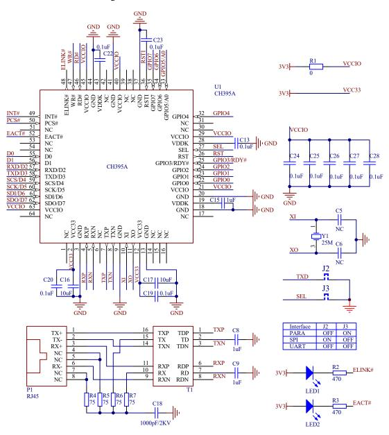
Figure 9-2 CH395A Hardware reference circuit
