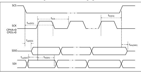
Figure 7-5 SPI mode 0 timing figure
