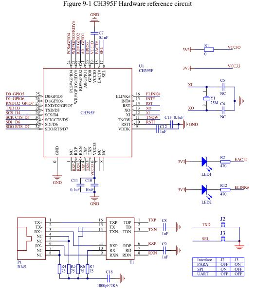
CH395F has built-in part of the oscillation capacitance of crystal Y1, C5 and C6 can be adjusted according to the crystal parameters. For Y1 with a load capacitance of 12pF, C5 and C6 are not required; for Y1 with a load capacitance of 20pF, C5 and C6 are recommended to be 15pF each.
