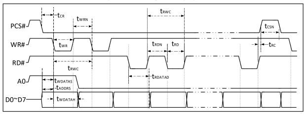
Figure 7-7 Parallel port timing figure
