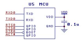
The image above shows the reference circuit that the MCU connect to CH343 through TTL to realize USB communication in dual power supply mode. VBUS is powered by CH343 through USB bus, the MCU and VIO use another self-powered VDD, which supports 5V, 3.3V or even 2.5V, 1.8V. When CH343 is connected with MCU, diode and other backflow prevention circuits can be omitted.
