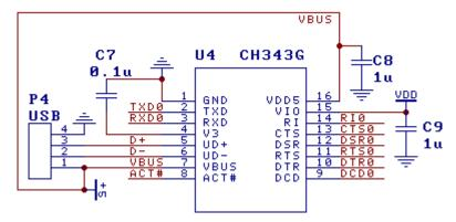
The image above is the USB to TTL converter realized by CH343G. The signal in the image can only be connected to RXD, TXD and public ground, while using the others as needed, all can be suspended when not needed.
