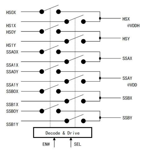
CH483M is uniformly enabled by EN# pin control and uniformly switched by SEL pin selection. The following table is its control table.
