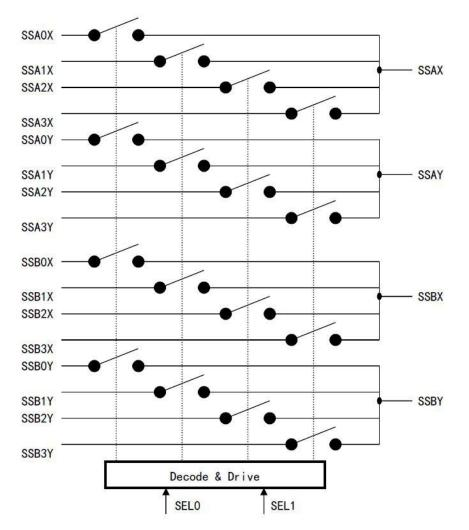
CH484M's channel is always enabled, and the switching of the channel is selected by SEL1 and SEL0 pins. The following table is its control table.
