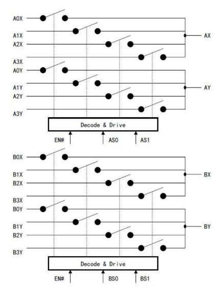
CH486F is uniformly enabled by the control of EN# pin, and the switch of channel A is selected by AS1 and AS0 pins, and the switch of channel B is selected by BS1 and BS0 pins. The following table is its control table.
