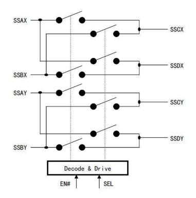
CH481D is uniformly enabled by EN# pin control and switched by SEL pin selection. The following table is its control table.
