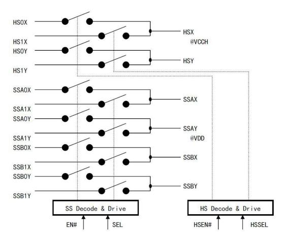
The SS of CH483X is enabled by EN# pin control and switched by SEL pin selection. The following table is its control table.
