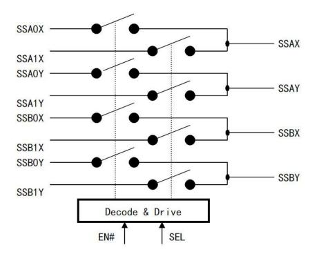
CH482D/X is enabled by EN# pin and switched by SEL pin. The following table is its control table.
