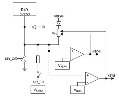
The default KEY\_OE=0, and the KEY open-drain output is prohibited. The default KEY\_PD=0, and only pull-up is provided. When KEY\_PD=1, the KEY outputs a weak low level of VREFM, which supports external P-type MOSFET gate control with a voltage not exceeding VDD49, and also supports key detection. KEYHI and KEYLI are input samples under high and low thresholds, and the pull-up resistance value is fine-tuned according to the results.
