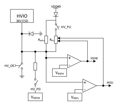
The default HV\_OE=0, and HVIO open-drain output is prohibited. The default HV\_PU=0, the default HV\_PD=0, and only the weak pull-up resistor RWPU is provided. When HV\_PD=1, the output  $V_{REFM}$  of HVIO is weak and low, which supports external P-type MOSFET gate control and key detection. HVHI and HVLI are input samples at high and low thresholds, and the pull-up resistance value is fine-tuned according to the results, and RPU pull-up is provided when HV\_PU=1.
