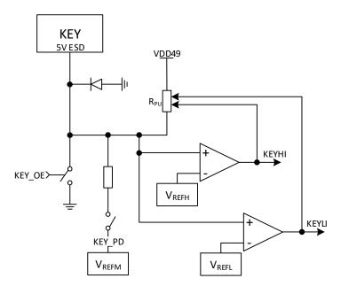
Default KEY\_OE=0, KEY open-drain output disabled. Default KEY\_PD=0, pull-up only. When KEY\_PD=1, KEY outputs VREFM weak low level, which supports gate control of external P-type MOSFET power tubes not exceeding the voltage of VDD49, as well as key detection. KEYHI and KEYLI are high and low sub-threshold inputs to be sampled, and the value of the pull-up resistor is fine-tuned according to its result.
