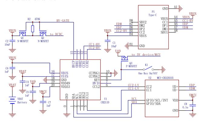
The CH211 provides Type-C Rd pull-down resistors for PDUSB MCUs (e.g. CH32X035 or CH32L103) that support PD Source, Sink, and DRP, and the HVCP pin generates a high voltage that can be used to control the DCDC on/off, charging the battery, or reversing the output. If it is used for Source only, then the 2 CCPDG pins should be dangling, and the VBUS pin of CH211 does not need to be connected.
