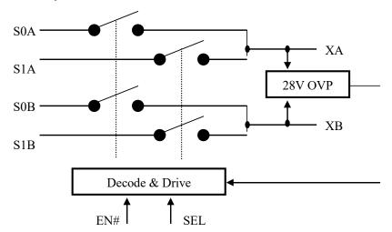
CH9442 is enabled or turned off by EN# pin control, and is switched by SEL pin selection. The following table is its control table.
